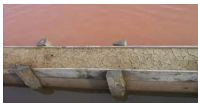
Picture 2: From a salt-pond in Slovenia. The wooden wall separates two chambers with different salt concentrations. The chamber with the strongest colour has the highest salt concentration. Photo: Taran Skjerdal, 2004
